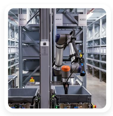
Assuming an average pick rate of 250 PPH per robotic picker and 25 PPH per AMR, a warehouse using a Goods-to-Robot system would need 4 robotic pickers and 40 AMRs to achieve a throughput of 1,000 picks per hour.
